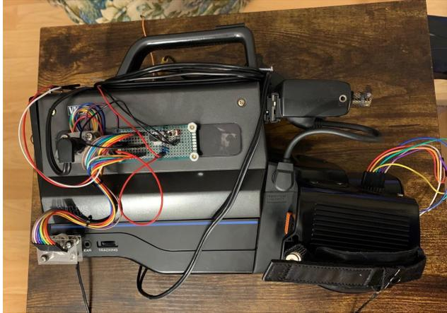
If you want to splice in another rca source take a normal rca cord, cut off one side of the adapter and strip the wires, soldering them to two female jumper wires.
