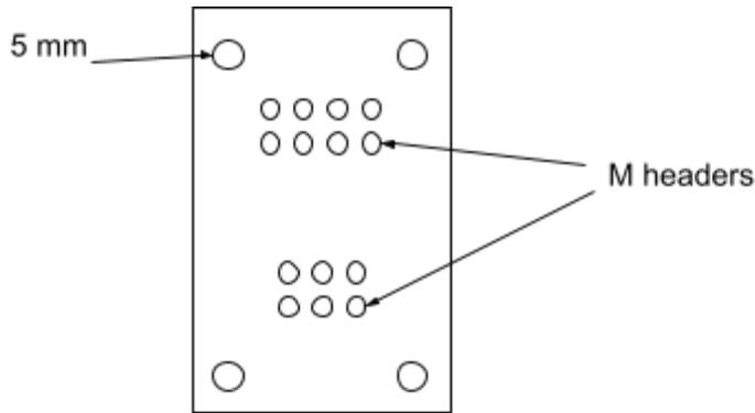
Lastly solder the wires to the headers on the circuit you just built. The wires from the camera port should connect to the bottom row of three headers in the order that they are labeled in the photos left to right. Same for the four wires from the chip.
