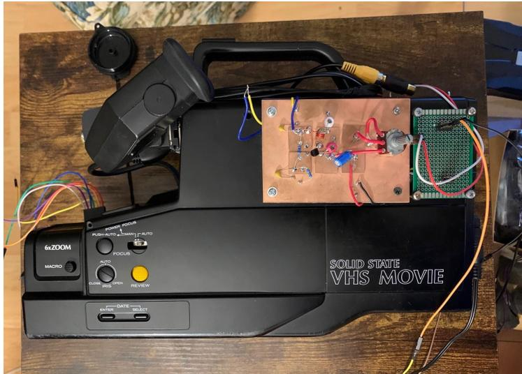
Once you build the tv transmitter you should attach the video input wires to two male headers and hot glue it to the side of the copper plate. This makes it easy to attach and detach it from the cord interface you built above.
