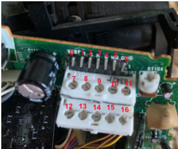
The top row is what we're mostly concerned with. Simply add jumper wires to these male pins. I explain how to get different color distortions in the use section. The two rows below that also allow color distortions but can be very finicky and difficult to adjust except through the use of a small screwdriver so I've left them alone in this version.
