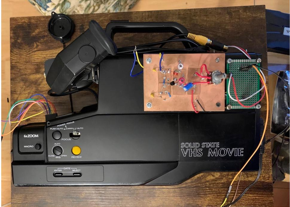
Now using a small perf board create the basic interface seen below.
