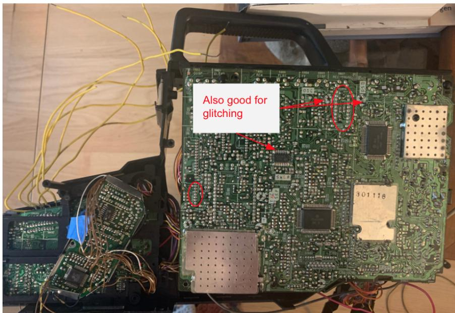
First solder thin gauge wire to the ports nearest the camera lens on the pins shown below to the left. Leave about a foot of loose wire. Then solder about 8 inches of thin wire to the chip below the rec/pause button on the points shown below on the right.
